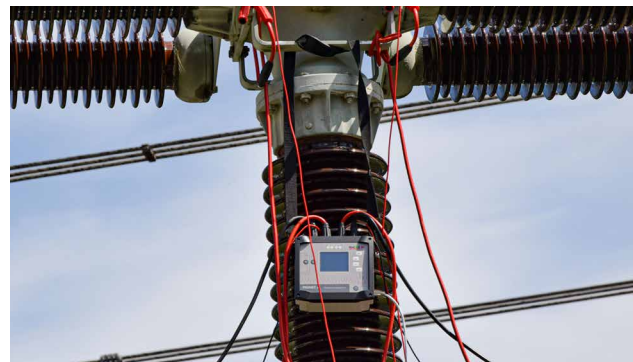
Figure 6: PROMET SE on a high-voltage breaker with two interrupter units.
