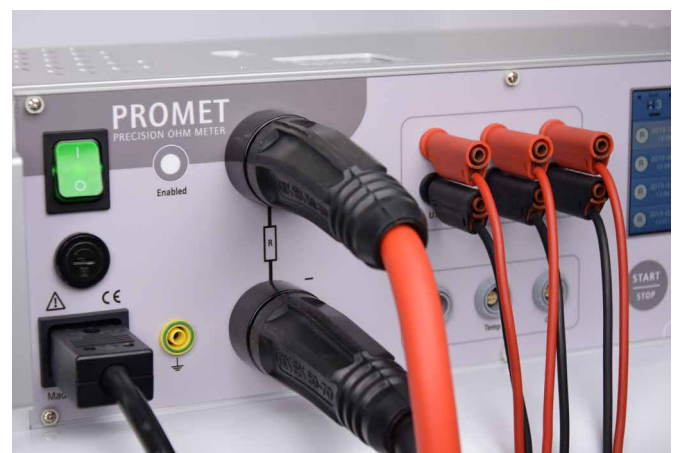
Four-wire connection to PROMET R300/R600
