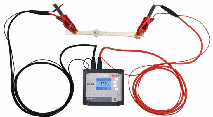
Measuring with PROMET SE and Kelvin measurement clamps
